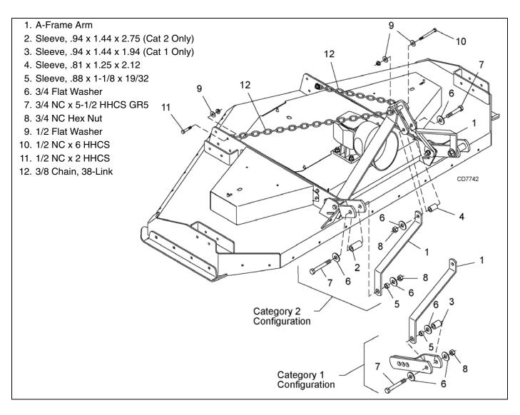
Figure 33. Quick Hitch Kit Installation (Optional)
